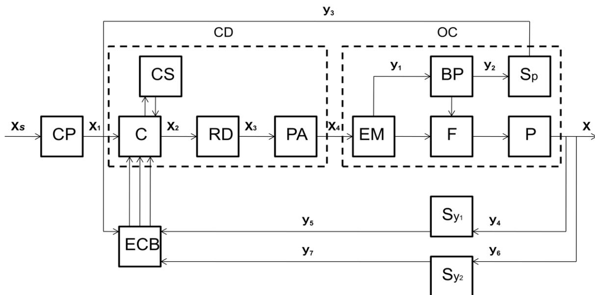
Figure 5. Functional diagram of the control system to upgrade the exercise bike
