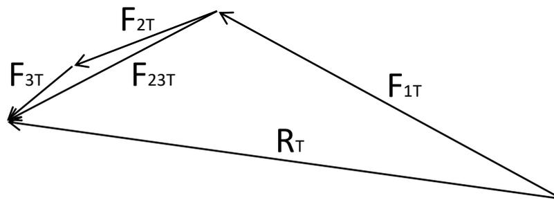
**Figure 4. Graphical definition of the resulting experimental muscle**
